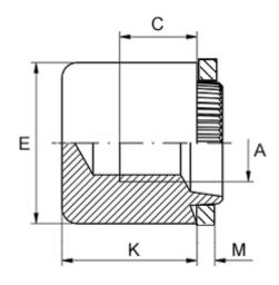
Female thread A = M5Height K = 10.0Min thread length C = 5.0Outer diameter E = 11.0Plate thickness = 4.1 to 4.3
